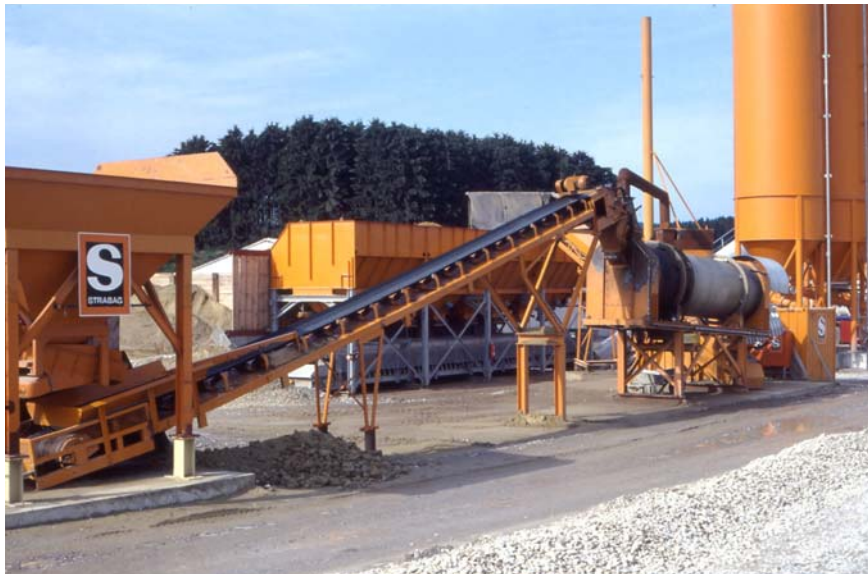
Photo 5: Mixing plant for mixed in-plant coarse grained well graded mineral liners
