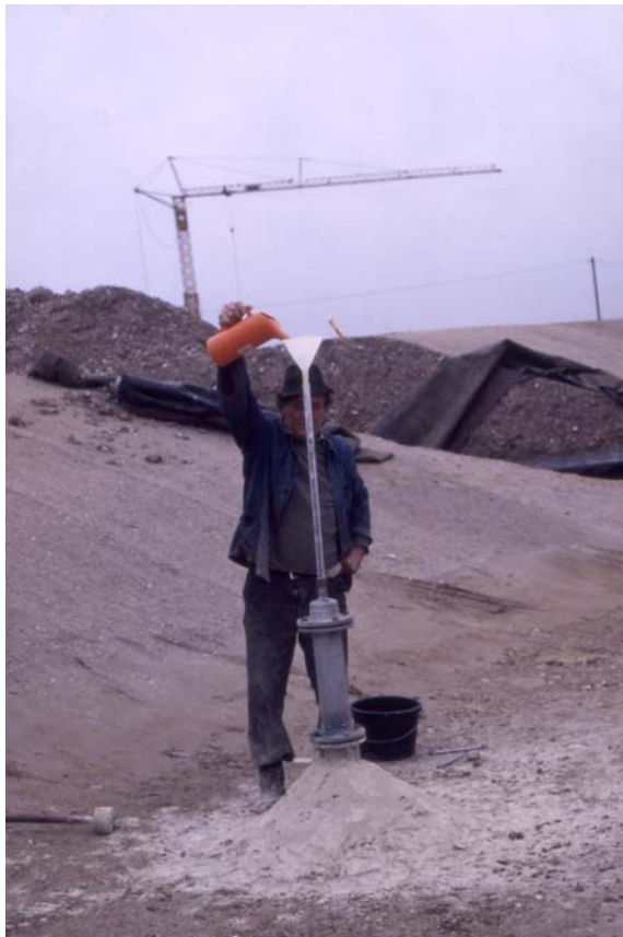
Photo 7: Infiltrometer for in-situ permeability testing
