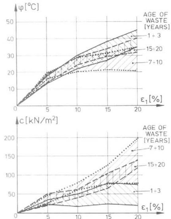
Figure 6: Deformation dependent shear parameters (JESSBERGER et al. 1995)
