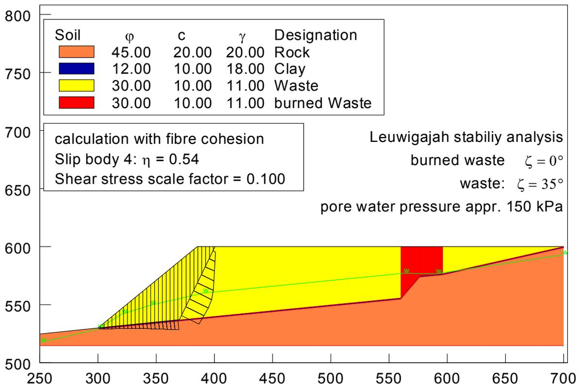
Figure 9: Stability analysis according to the common method
