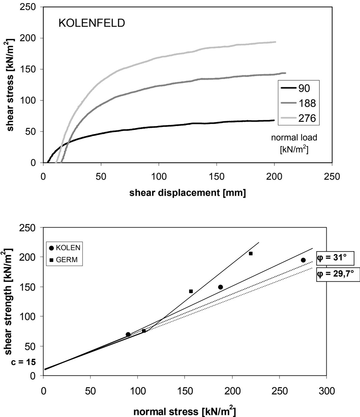
Figure 4: Direct shear test on MSW – results: stress-strain (left), non linear shear planes (right)
