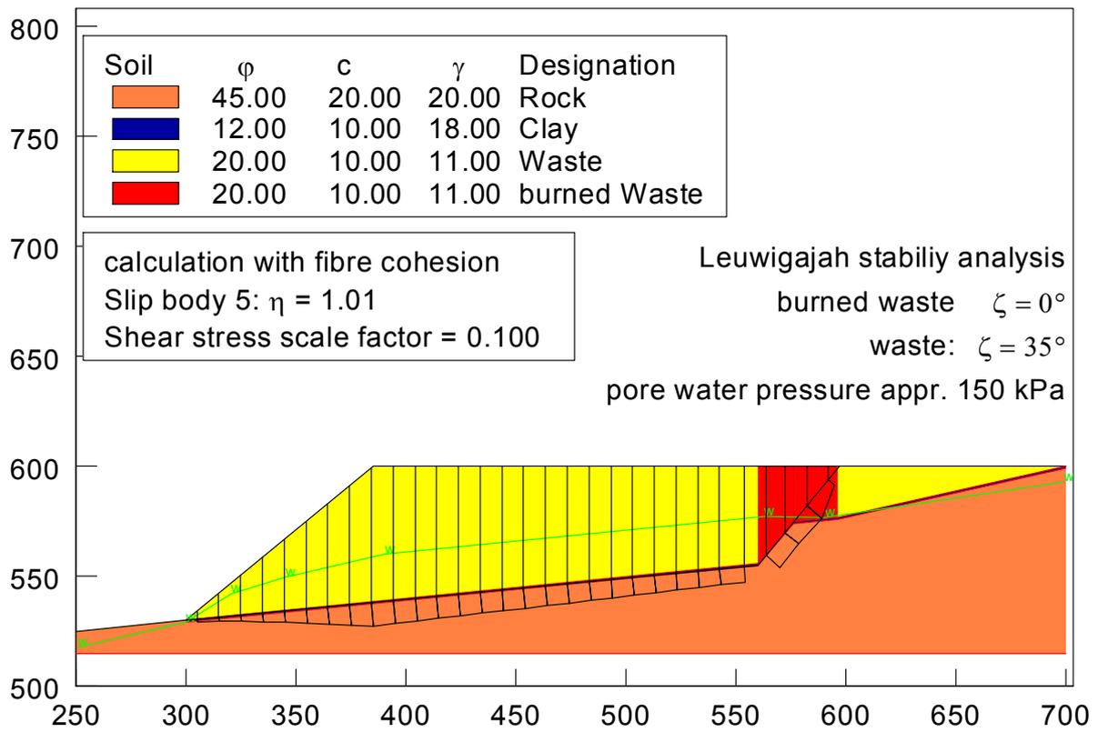
Figure 8: Stability analysis according to the advanced method of fibre-cohesion
