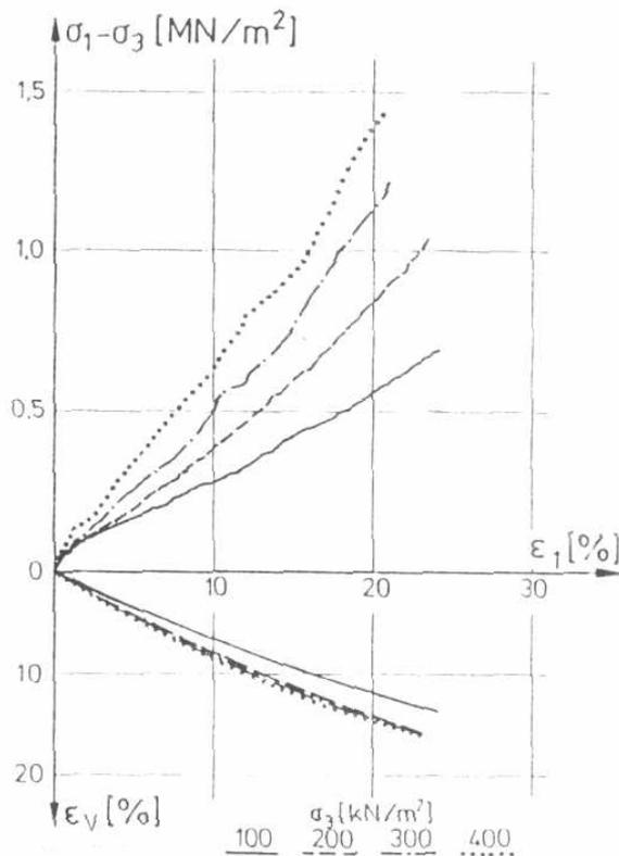
Figure 5: Results of triaxial compression test (JESSBERGER et al. 1995)
