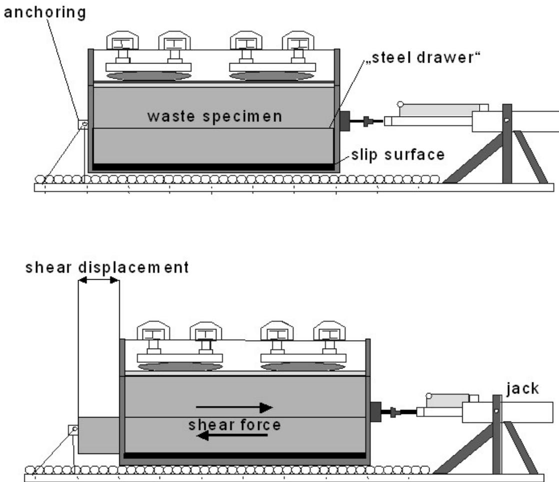
Figure 3: Large shear test – testing procedure
