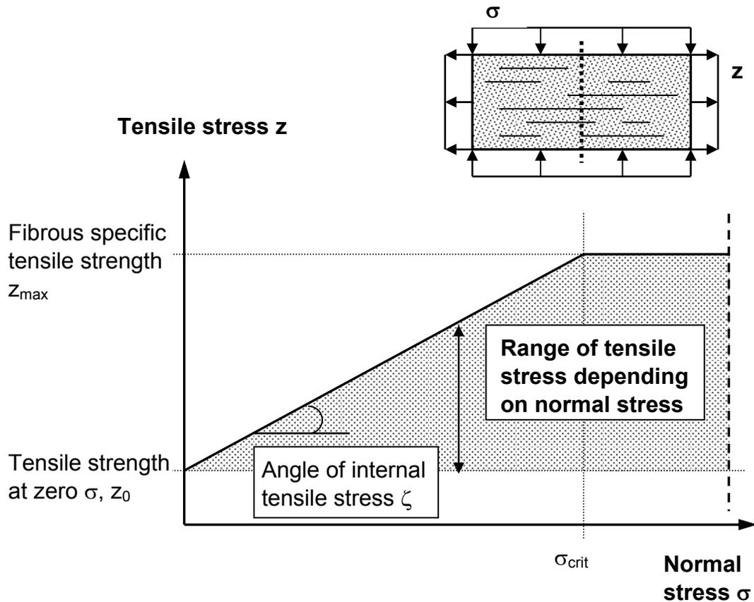
Figure 1: Failure characteristics of fibrous waste material in tension test under normal load
