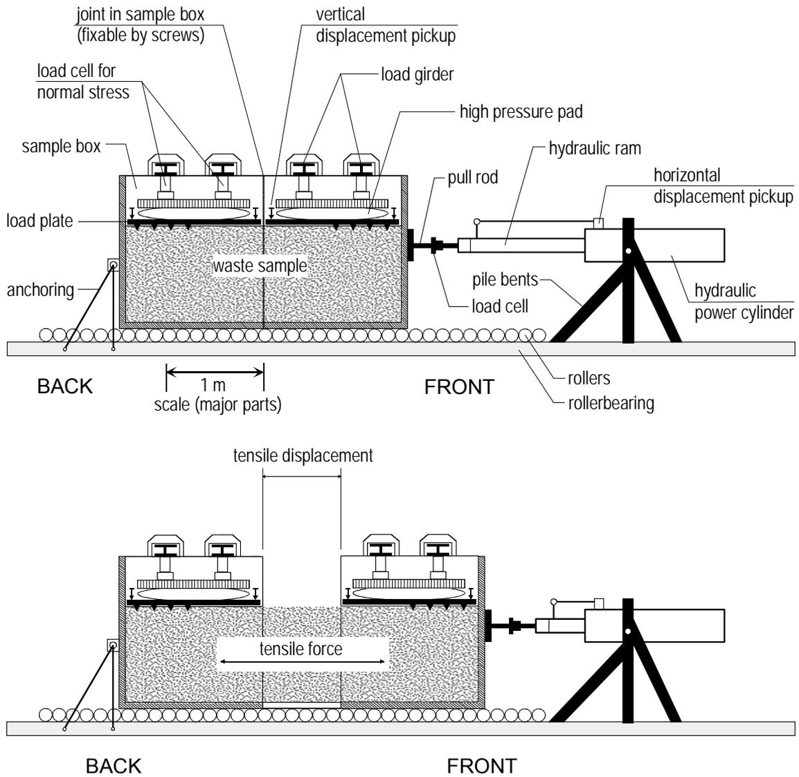
Figure 2: Tension test under normal load – principle and procedure
